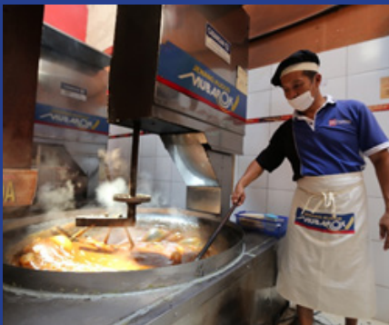
One of the supporting facility that's made: mixer for jenang dough.
